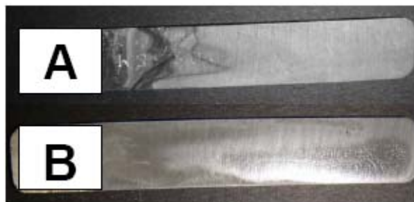
Figure 45. Phenomenology of the anticorrosive effect of Ca-PBTC films on carbon steel. The upper specimen is the “control” (A), no inhibitor present. Surface “cleanliness” in the lower specimen (B) by a 1 mM \text{Ca}^{2+} /PBTC synergistic combination is demonstrated, but metal loss is enhanced (see text)
