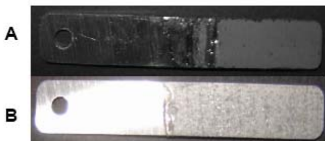
Figure 43. The anticorrosive effect of Zn-HDTMP films on carbon steel. The upper specimen is the “control” (A), no inhibitor present. Corrosion inhibition in the lower specimen (B) by a 1 mM Zn^{2+} /HDTMP synergistic combination is dramatically demonstrated
